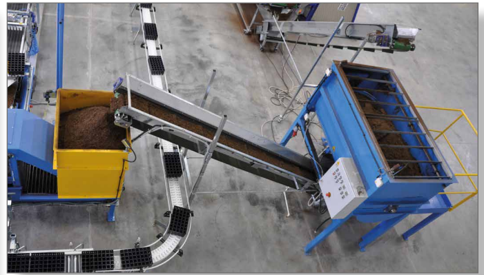
Open top and operator's platform allows monitoring of the process.
